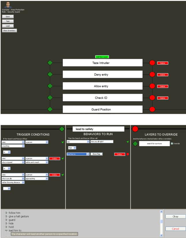
Fig. 1. The BehaviorShop game AI behavior designer is a subsumption-based editor for creating controllers for game characters. The top image shows the subsumption editing screen, which allows the user to create new layers and rearrange existing layers through a drag and drop interface. The lower image shows the layer edit screen that is used to fill in the details, including the behaviors and triggering conditions, for individual layers.
